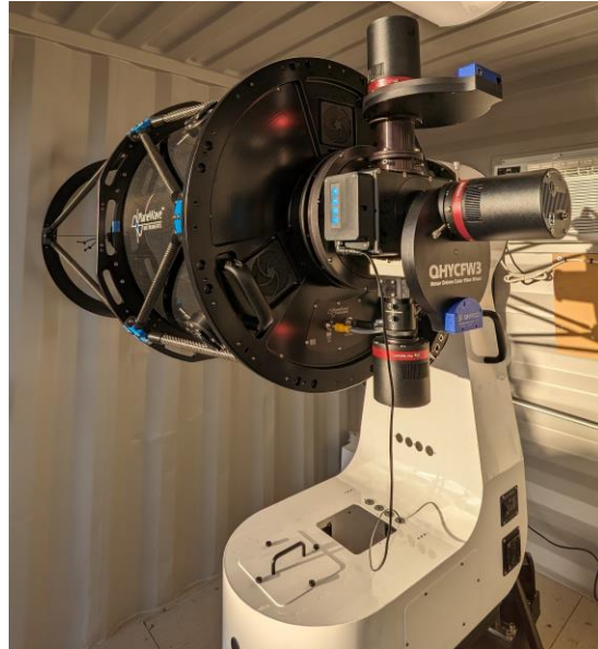
Figure 7: The fully instrumented PlaneWave Instruments CDK-500 telescope in its initial Conex shelter.
