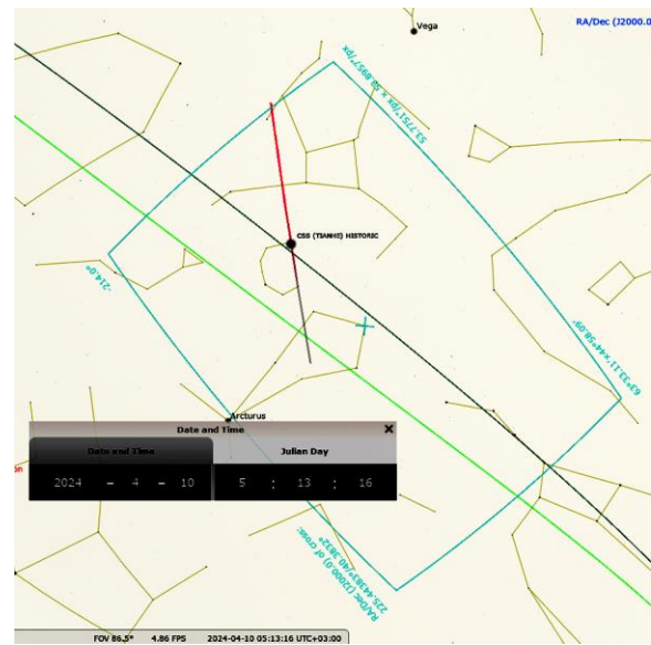
Figure 1. Stellarium chart showing the track of the Tiangong amongst the constellations during the pass (negative, or inverted display). The blue rectangle is the Canon 500D sensor field of view (FOV). The light and dark green curves crossing the field from bottom right to top left are the umbra and penumbra of the Earth, respectively. In red, the segment of the satellite track from its exit from the umbra to the field edge (compare this view to Fig. 4).
