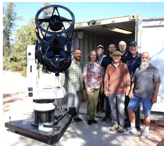
Figure 1: Initial roll-out configuration features the PlaneWave Instruments 0.5-meter telescope on a rolling pier. The telescope is stored in the Conex shipping container when not in use on the Payson campus.
