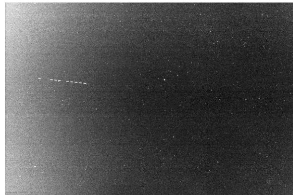
Figure 5. The second 10-image burst, commencing at time T02:14:40:07 (Set 2). Notice a defect in the stacking at tracklet #6 (barely visible) and the delayed image of the 10 th tracklet at far left. The length of the tracklets is smaller than in Fig. 4 due both to increased range ( \sim 750 km) and perspective. The bright star just above the center right is Altair ( \alpha Aql).
