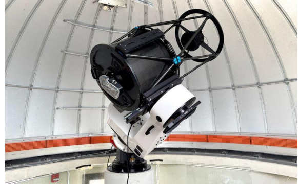
Figure 8: A PlaneWave Instruments CDK 500 telescope on an equatorial wedge under a 16-foot Ash dome at the King's Academy in Jordan. This is very similar to the final Richard F. Caris Observatory's configuration.
