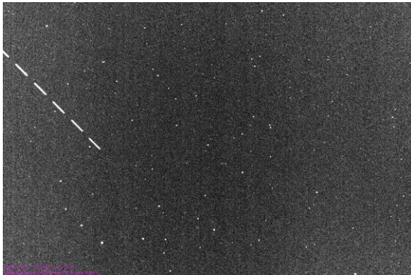
Figure 4. The first 6 tracklets of the 10-image burst commencing at time T02:13:11:61 (Set 1). Notice a defect in the stacking at tracklet #1 (barely visible). Corona Borealis is visible at the bottom left. The initial range is \approx 390 km.
