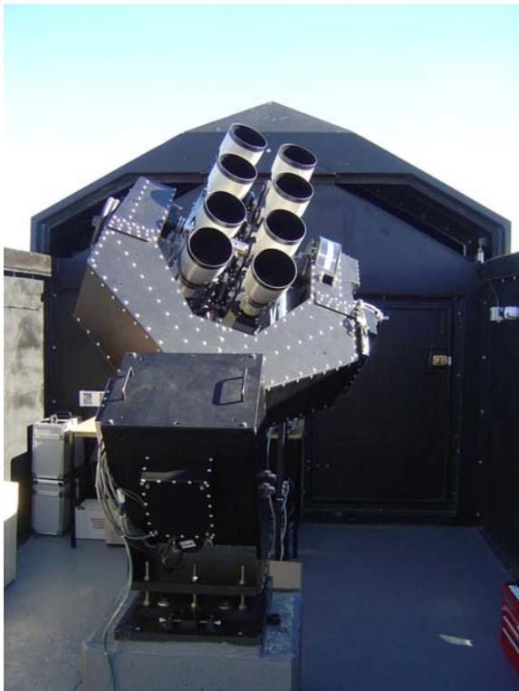
The SuperWASP cameras. The TORUS fork mount supports 8 identical Canon 200mm f/1.8 lenses (11 cm aperture). Each CCD is a 2048 x 2048 thinned e2v camera produced by Andor Technology (photo credit: David Anderson)
