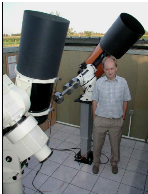
Figure 1. CBA Belgium Observatory, one of the nodes of the CBA network, is remotely operated by Tonny Vanmunster. It features two CCD-equipped 0.35-m telescopes on computerized mounts
