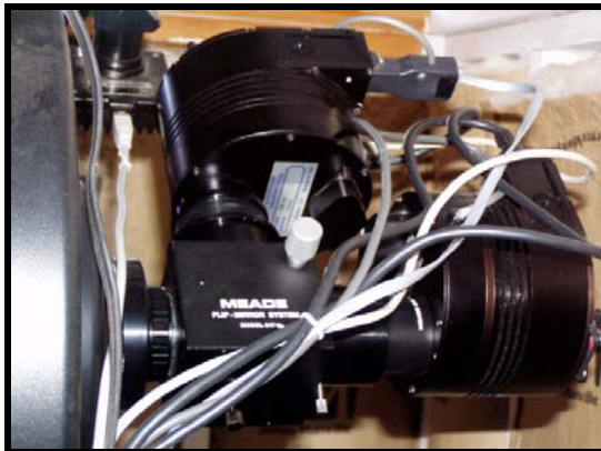
Figure 3. This is an overview of the two-channel test-photometer. The Meade 14-inch LX-200GPS telescope is on the far left. Coupled directly to it is the Meade 2” flip mirror system. The f/6.3 focal reducer and SBIG ST7XE camera and filter wheel are shown in the upper middle, while the SBIG ST8XE camera and filter wheel are shown on the right.
