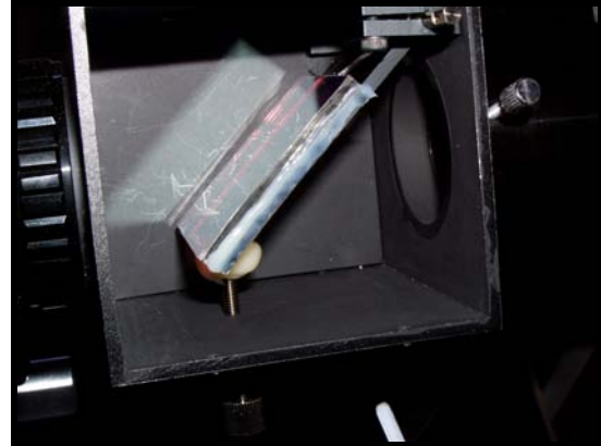
Figure 4. This shows the Edmund Industrial dichroic filter which replaced the mirror in the Meade flip mirror system (with the system’s side cover removed).
