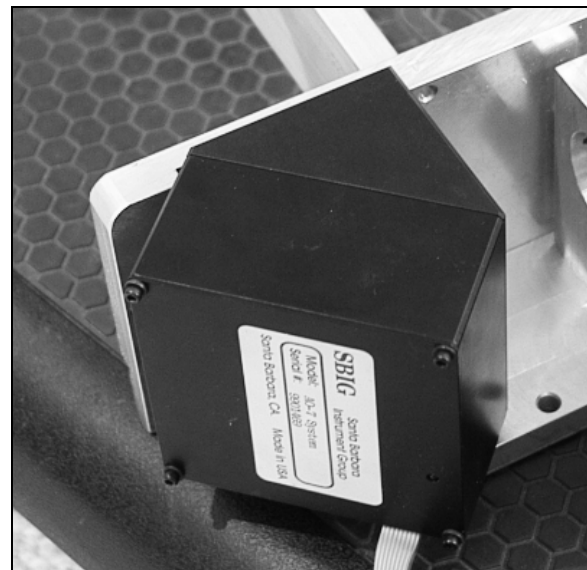
Figure 10. The AO-7 from SBIG provides fully scriptable control of the tip / tilt mirror. This can be used to step scan an image with a single pixel detector.
