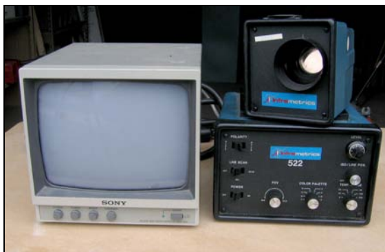
Figure 4. Inframetrics produced this mid-IR imaging system in the 80's. The MCT sensor has a range out to 14 microns and can display video in false color as well as black and white.
