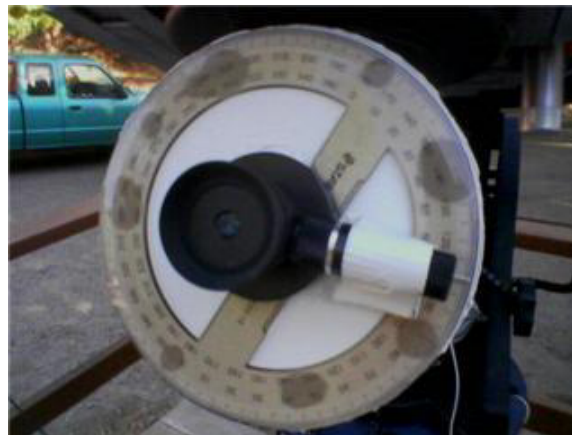
Figure 2. A protractor-pointer designed by Johnson to measure the position angle of the double star STF 2079.
