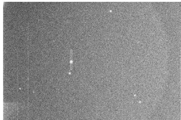
Figure 5. After 60 minutes of guiding, star UV Tau is still centered on the slit.
