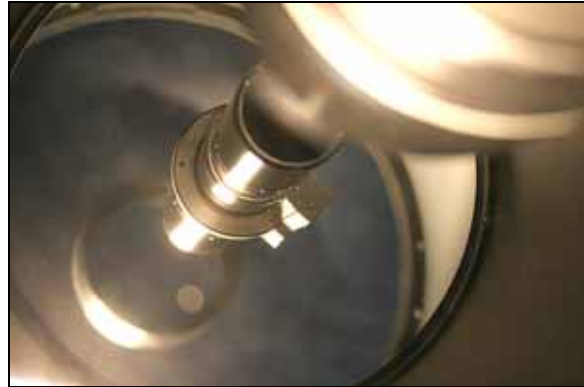
Figure 7, Two-Pair Magnetic Loader Installed on C14 Optical Tube
