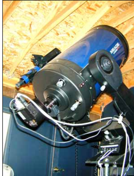
Figure 3. Meade 14” LX200GPS with SBIG ST-7E Camera attached.
